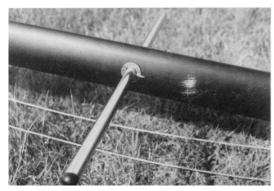
**5**. To assemble the diamonds on the lower mast section, first untwist the wires, then insert the spreader tube, slip a washer on each side and push the cotter pins through the holes in the tube. Bend over the cotter pins so they will not fall out. Note that the washers are between the cotter pins and the mast.
