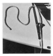
**2**. Note that the ropes from the rigging board are secured in the cam cleats of the jib fairleads.
