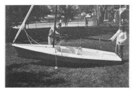
**32.** The first time you rig your boat, have your crew hold the end of the boom level to the ground and make sure the boom yang and mainsheet ropes are correctly reeved before hoisting the sail.
