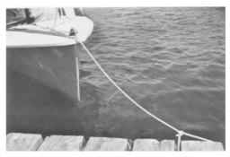
Check and tighten all inspection hatches. Tie a painter to the bow fitting which can be left in place while on the water.
