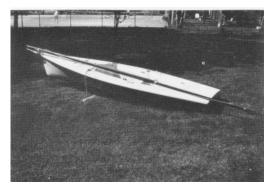
11. Place mast on deck with foot facing forward and leading edge up.
