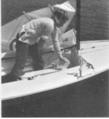
**54.** Make sure the carpet in the centreboard box is clean, dip the centreboard in water to lubricate it and insert into the box as shown making sure the cut-off corner at the top is forward. Put it down as far as you can as it will help prevent the boat rolling from side to side while hoisting the sail. If the water is very shallow, however, leave it out until you leave the dock as it will get in the way while hoisting.
