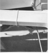
**43.** A useful method of carrying the halyard tail is to make a loop of shockcord around the centerboard capping. Use this to carry a sponge for cleaning up the boat and carry your halyard tail under the capping between sponge and shockcord.
