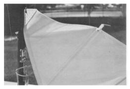
**38.** Shackle the halyard to the headboard and start the bolt rope into the groove of the mast. (On most early boats the sail will have to be started into the groove before attaching the shackle. The halyard was made shorter so that the sail head would always stay attached to the mast when lowered.) Note that the mast rotation lever is lowered flat against the mast to permit easy access to the bolt rope groove.
