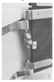
To remove, simply depress the spring and lift.
