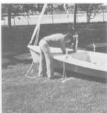
**19.** Slide this hand onto the deck just forward of the mast pin. The mast won't fall over in this position and you can now take your time placing it over the pin with both hands. If the mast does not go over the pin it is because the stay slides are not all the way forward or there is a kink in one of the three wires holding up the mast.
