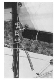
Finally rigged, it will look this way. All adjustments to either tighten or ease the tension on the luff of the sail can now be made at the black clam cleat below the gooseneck.
