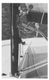
**42.** When the halyard is locked at the top of the mast, pass the loop of the shockcord under the small black hook and remove the rope tail completely.
