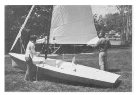
**40.** When the sail is nearly at the top, lift the boom off the gooseneck pin; it helps if one person holds the boom up to take its weight off the sail. Loosen the vang, because if it is tight, it will hold down the end of the boom and raising the sail to the top will be impossible.
