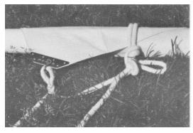
**13.** Attach the jib sheets with the shackle provided (use the hole second from the top to start with) and use one end to tie a loop around the rolled jib to prevent it from unfurling while raising the mast later.
