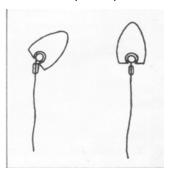
It also helps if the mast is aligned exactly in the direction of the sail so that the batten protectors do not bind on the back of the mast. Make sure the boom vang is slack and not cleated.
