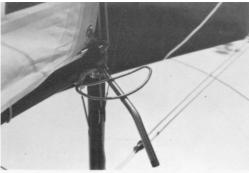
**48. When sailing on any other course** (ie reaching or running), lower the lever slightly and rotate it even further. Then raise it and lock it behind the plastic stop as shown in these two photographs taken from opposite sides of the sail. This is important as the mast will usually flip out of rotation (only annoying, rather than anything else!) as soon as the mainsheet is eased for reaching.
